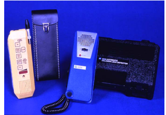
HFC Leak Detectors
